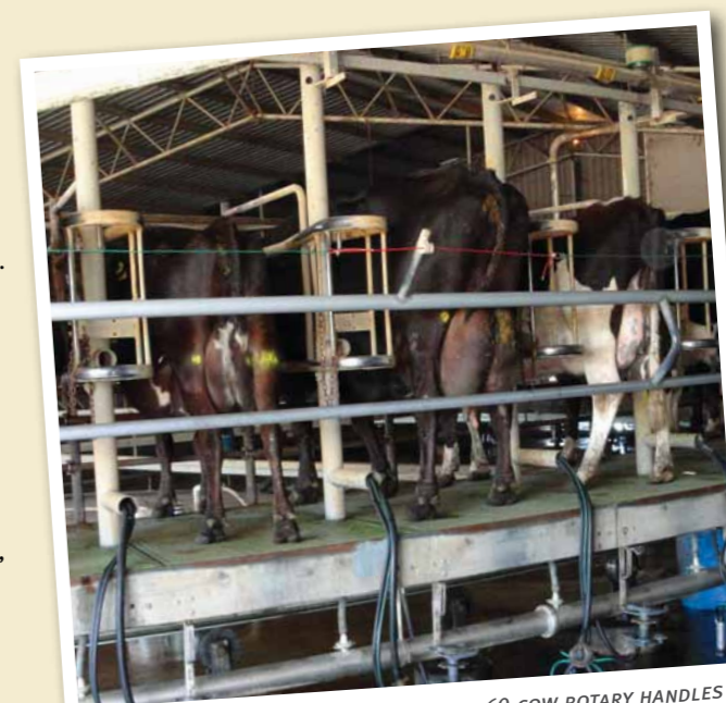
THE WHITE'S IMMACULATELY MAINTAINED 60-COW ROTARY HANDLES THE MILKING IN A MAXIMUM OF THREE HOURS.
